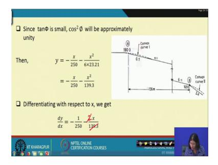
So down to this form of the equation it is a quadratic equation; now since we are dividing the channel reach into small small section, so, we differentiate y with respect to x.
