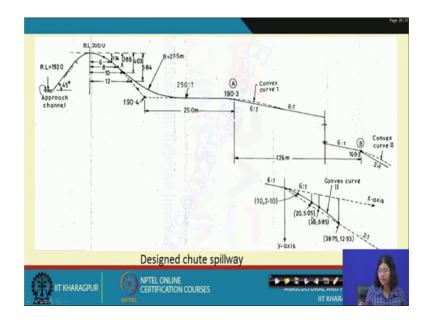
So, this is the complete design. So, first we designed profile this one and then the control structure or the ogee where. And then we sorry then we proved the convex curve here that is slope of 6 is to 1 and first convex curve and then we provide a second convex curve that is 6 is to 1. And this is the curvature and the slope of this convex curve is shown here. So, this completes your design chute spillway.
