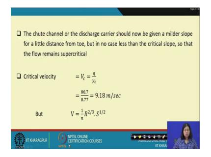
The chute channel or the discharge carrier should, now be given a milder slope for a little distance from the toe, but in no case this should be less than the critical slope. So, the flow remains to be a supercritical then the critical velocity V c is q the critical discharge divided by y c, which is the critical depth.
