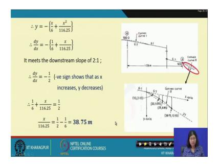
And we the equation and then after getting y value we differentiate with respect to x here. So, it meets the downstream slow at slope of 2 is to 1 and since d y by d x is minus 1 by 2 we solve it like this.
