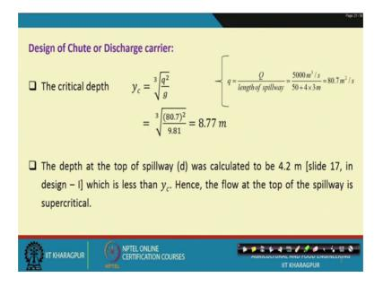
So, here we designed the component 3 that is chute or the discharge carrier; that is one of the component of the chute spillway. So, here we have to calculate the critical depth; so, critical depth is calculated using the discharge of the spillway and the length of the spillway using this equation.
