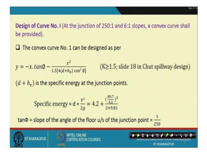
Now, the design of curve number 1 at the junction of 250.1 and 6 is to 1 slope since the slope is now from my steeper to milder, a convex curve shall be provided. So, the convex curve is designed as per the equation. So, this was the equation given earlier and K is assumed as 1.85; so, which is also given in slide 18 in chute spillway design part 1.
