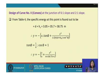
Now the design curve number 2 at the junction of 6 is 1 slope and 2 is to 1 slope. From table 4 the specific energy at this point is find out to be d plus h v that is 38.75 metre. Now since tan phi is 1 by 6 the cos phi is approximately 1; so, y equal to minus x by 6 with plug everything here.
