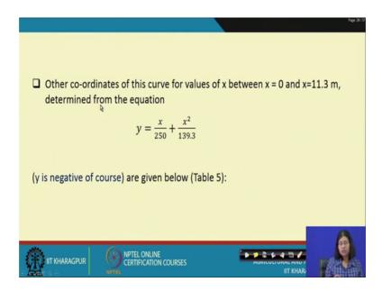
So, other coordinates of this curve for values of x is between 0 to 11.3 metre is determined based on this equation; so, y is negative of course as given below in the table 5.
