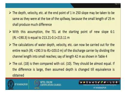
So, at the depth velocity etc at the end point of 1 in 250 slope maybe taken to be same as they were at the toe of the spillway because the small length of 25 metre shall produce a
