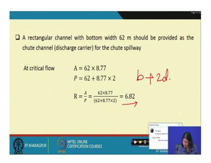
So, a rectangular channel with bottom width of 62 metre should be provided a chute channel for the chute spillway. So, at a critical flow; so, this is the area of the channel, so, b into d.
