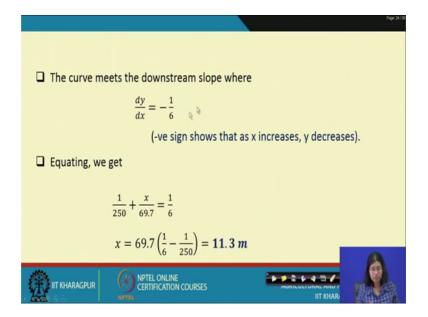
The curve meets the downstream slope where d y by d x is minus 1.6; the negative sign shows that as x increases the y also decreases. So, we plug it here sorry this; this thing will be 2 x it is a small correction. So, it will be 69, 68 point something there is a small correction here please note. So, we plug it everything here and we get the value of x as 11.3 metre.
