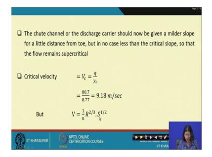
So, we everything plug going to plug here into the equation. So, we calculated the weighted perimeter and the area of the channel cross section.
