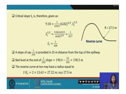
So, now the critical slope we like this we calculate the critical slope here. So, which is 1 upon 428 it is a reverse curve a slope of say 1 upon 250 used to be provided at a 25 metre distance from the top of the spillway. Since the critical slope is come out to be 1 upon 428, so we gave a distance of 25 metre at the top of the spillway and then we provide slope of 1 upon 250. So, bed level at the end of this slope is 190.4 from earlier
