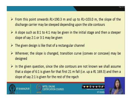
Now we have to construct a table for the design problem. So, from this point onwards relative level of 190.3 metre and up to relative level of 103 metre; the slope of a discharge carrier may be steeped depending upon the site contour.
