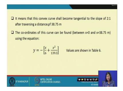
It means that the convex curve shall become a tangential to the slope of 2 is to 1, after traversing a distance of 38.75 metre. The coordinates of this curve can be found out from
