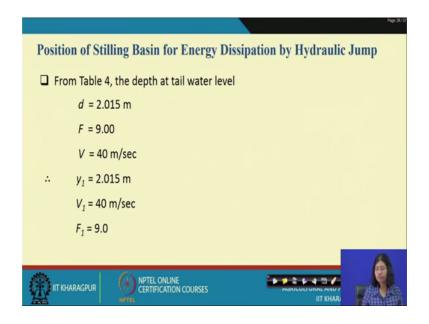
Now the position of the stilling basin for energy dissipation by hydraulic jump from table 4 the depth of the TEL water level. So, d equal to 2.015, F is Froude number and F 1 is 9 metre.
