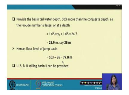
So, provide the basin tail water depth 50 percent more than the conjugate depth; conjugate depth as we remember y 2 and y 1 both as the Froude number is large at a depth 1.05 into y 2.
