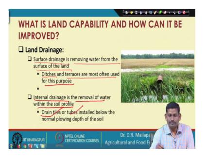
So, the next is the land drainage so, land drainage vertical basically the surface drainage removing water from the surface of the land. Generally, ditches and terraces are most often used for this purpose. And then there is a internal drainage. So, this is the surface and this is all subsurface drainage we can say, it is removal of water within the soil profile.
