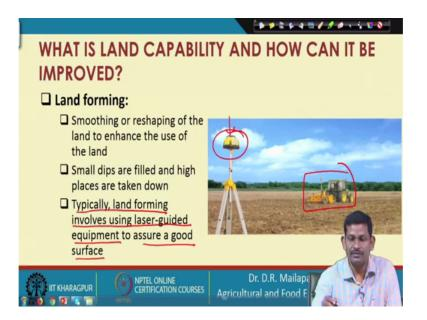
So, the typically the land forming involves using a laser guided equipment to assure the good surface so here if you see laser guided equipment. So, this is a tractor so, which shapes the land. And here this is the laser guide so, it guides the tractor where to you know remove the soil excess oil and where to add that excess soil so that the desired you know grade can be achieved.
