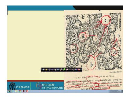
These are ice crystals right, a like this, these are ice crystals right then b is air cells, these are air cells right. These are air cells and, then c is unfrozen material, whatever is not frozen that part is c. This is that c is the unfrozen material right and another thing which you need to know is that let me take it temporarily to this side, because, temporarily I am taking it ok.
