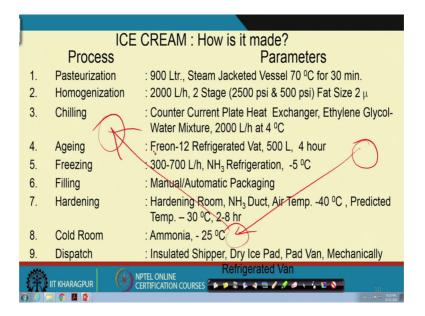
It is so big a distance that here, if it is produced here, if it is to be consumed may be in between one cold room is there. So, it comes here stays there for days together and maybe depending on requirement is goes to there right. So, this way the ice cream is manufactured in the, this is the process flowchart and the parameters, which are involved in the production right.
