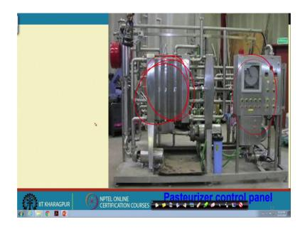
This is for the a of, laboratory use our thing. So, this is the pasteurizer right and then it goes to homogenizer. So, this is a pasteurizer with these. These are the plate; this is the plate heat exchanger. So, with the controls and other things, all pipelines, this is the commercial one. So, pasteurizer are using for pasteurizations plate, plate heat exchanges. Then it goes to, then it goes to homogenizer.
