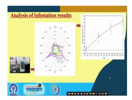
In this slide that it is the e-nose which we have the sensor data. Then it gives the radar charge there are e-nose which we have; it has 18 metal oxide sensors. So, these sensors
