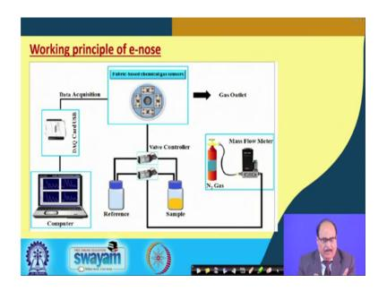
So, accordingly the working principle in the same manner as I told you that is the there is a some nitrogen or some other gas, whether the samples broken or evaporated, then the samples components in the form of vapors are taken. And these vapors are sensed by that volatiles, they are sensed by the different sensors and the data is sent to the computer.
