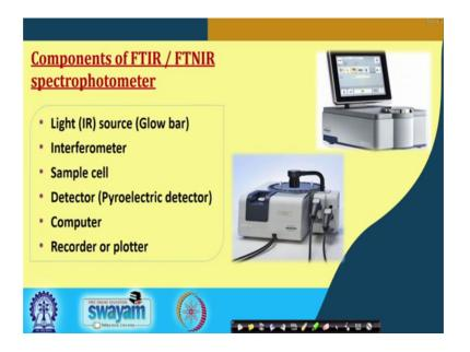
So, accordingly the components of an FTIR or FTNIR spectrophotometer includes that is a light source glow bar, an interferometer, a sample cell, then a detector, computer, and recorder or plotter. So, this is one FTNIR system which we have in our laboratory or FTIR system etcetera that is the simple it is very simple and handy instrument which can table top instrument, and it is compact system that is computer. In this case, the computer is connected separately.
