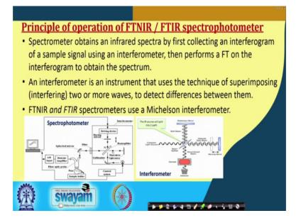
Principle of operation of FTNIR or FTIR is spectrophotometer that is as you can see in this picture. It is there are spectrophotometer are provided by some interferometers. So, a spectrophotometer obtains an infrared spectra by first collecting an interferogram of a sample signal using an interferometer, then it performs Fourier transform on the interferogram to obtain the spectrum.
