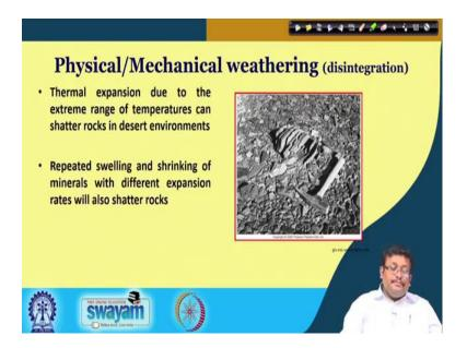
So, we call it frost wedging. Not only that, the thermal expansion due to the extreme range of temperature can shatter the rocks in desert environment, where there is an extreme climate and extreme temperature events can occur. For example, in the desert area, you will see that in the daytime there is a high you know very hot environment; however, in the night the air gets very much cold.
