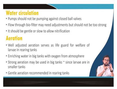
So, water circulation. How the water circulation should be controlled? The pump should be should, the pumps should not be the, should not be pumping against the closed ball, closed ball valves. Definitely you have to make sure that all the valves are open and so that how you can ensure it. So, you can check the arrow sign over the this valves and this all this closed ball valves.
