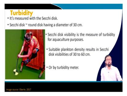
So, in general, it is measured using the Secchi disk. The Secchi disk is around the round disk, you can see this lady is holding a disk, this different colored, this two-colored disk, where it's normally it has a diameter of around 30 centimeter and it actually gives you the visibility as a measure of turbidity for aquaculture purposes.
