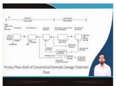
This is the process flow sheet of a conventional domestic sewage treatment plant. Here I will mainly be focusing on sewage treatment plant rather than aquaculture treatment plant in the
