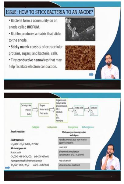
In the anodic biofilm, see this is the electron transfer mechanism that is happening because of the respiration process that is happening inside this specific type of microorganisms which we call electroactive microorganisms or electrogens, so what they do they utilize the food or nutrient and they excel they let excess electrons and all.
