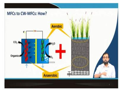
Now, so what is my constructed wetland microbial fuel cell? Microbial fuel cell, we discussed in last presentation last lecture right, it is very important; try to understand, you try to remember. In microbial fuel cell we have anaerobic chamber, which is anodic chamber; aerobic chamber, which is the cathodic chamber. What is happening in the anodic anaerobic chamber? The anaerobes, exoelectrogens, a specific type of microorganisms, which can grow there in the over the anodic surface.
