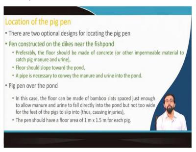
Location of the pig pen, there are two optional designs for locating your pig pen or the structure where we are actually being cultured. The pen constructed on the dikes near to the fish pond preferably the floor should be made of concrete or some impermeable material to catch the pig manure and urine and floor should slope towards the pond so you can simply wash it thoroughly and it will directly go to the pond, there will be some outlet point from which it will directly go to the pond.
