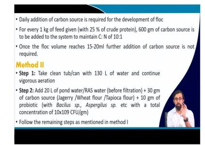
So, once you transfer to the main tank do not forget to provide them with the carbon source every day. For every 1 kg of feed given say like 25 percent of crude protein, 600 grams of carbon source is to be added to the system to maintain the carbon to nitrogen ratio of 10 is to 1. 1 kg of feed that you are supplying with say like 25 percent crude protein just to give you one example.
