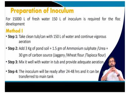
So, in order to give you an idea or the example of how it works, how to design or how to prepare the inoculum, so I am giving you one very specific example like with these two different methods. First one, say you have a 15,000 litre of fresh water which needs to be supplied with 150 litre of inoculum, at least 1 percent of it.
