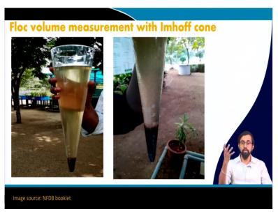
In general, this floc volume we can measure it using this Imhoff cone, this is a very standard practice by which you can measure or you can just simply do it by yourself also, but in general, this is the standard this Imhoff cone that we normally use for the floc volume measurement.
