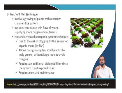
Nutrient film technique, it involves the growing of plants within a narrow channel of like gutters or like normal pipe like structure. So, in this pipeline structure, there is a narrow water body which is like keep on flowing and this water line of plants are placed at a certain interval. It includes a continuous this thin flow of water supplying more oxygen and nutrients and which will help the growth of the root much better way.
