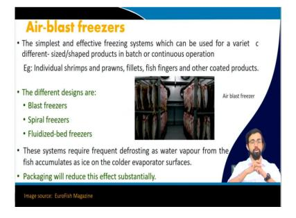
So, how does air blast freezing works? It is one of the simplest and effective freezing systems which used like different varieties of shaped products in a batch or in continuous operation. You provide this air blast and some at very low cost, low temperature and all. It will be used for individual shrimps, prawns, fillets, fish fingers and other coated products also.
