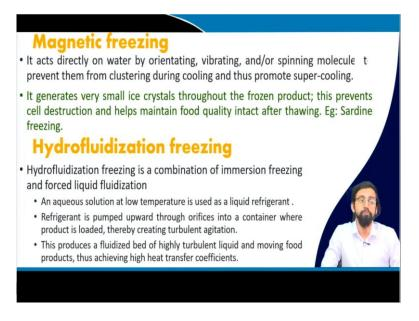
What are the other type of freezing methods? Like the magnetic freezing. What we are doing here the magnetic freezings, they the water molecules, all the molecules they constantly in a different state of locomotions. We call them orientation like in a vibration state, spinning states and all. So, all these things like this transitional and all.
