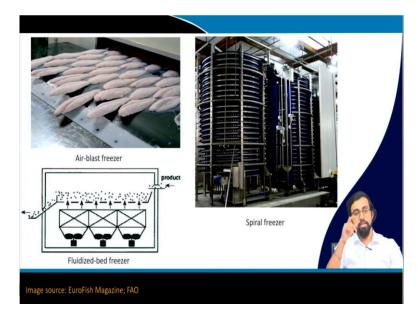
See this air blast freezer. I told you this conveyor belt it is coming out of these systems and it becomes very solid in nature and because of all the moisture present in its body is converted into ice. The fluidized bed freezes. You can see the air, the cold air is flowing from the bottom and because of its like it is a fluidized condition. So, why is a fluidized condition?
