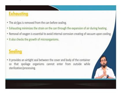
Second is called exhausting. What is exhausting? It is the process by which we can remove the gas or the air that is present in the can before sealing, before the final sealing, you seal the can. This exhausting it minimize the strain on the can through the expansion of the air through heating. It removes the oxygen which is essential to avoid any corrosion creating vacuum upon cooling.
