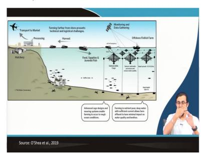
So, in general, you can have this advanced case designs and systems which can have a proper monitoring and the data gathering unit. It will be having underwater cameras and underwater sensors which will keep on giving you the real time data from your processing unit is from your system office itself.
