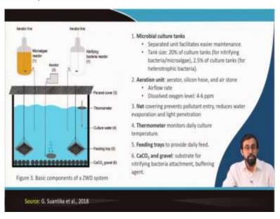
So, in general this is a very standard practice that you see in this standard practice in this standard method that is given by Suantika et al., 2018. You see the aerator line is given in each of the segments like say it has like four segments, first reactor is nitrifying bacteria reactor, second is micro algae reactor, fourth is this the whole tank itself where the cultured water is there, fifth is this aerators are there.
