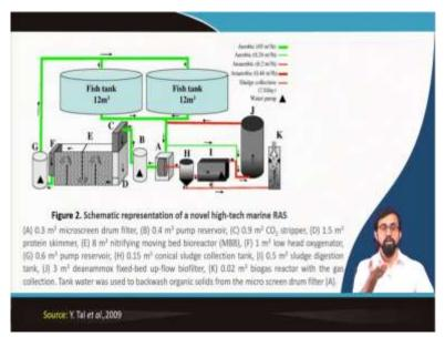
You can see this is another typical example of high-tech marine recirculatory (())(9:53) aquaculture systems, where you can see the fish tank, both of the fish tanks having 2 cubic meters of volume. Where the water which is coming out of the fish tank is introduced to the unit A, and B if you can see the first the microscreen drum filter from there to the pump preserver, that arrow sign is showing it means the pump.
