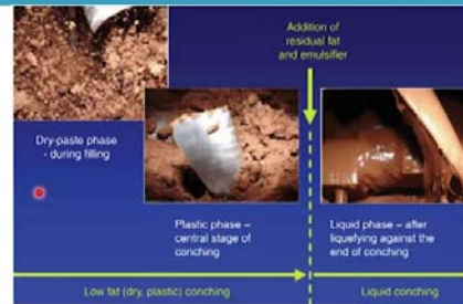
Different phases of the conching process
