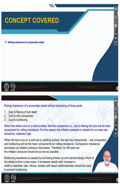
Now, here the concept will be how to find out rolling resistance of pneumatic wheel. So when you consider wheel, rolling resistance it will be because of three things, one is due to flexing of tyre, the other one is due to soil compaction and the rolling resistance could be due to bulldozing. So either all three are present or any one of them will be present so both will, that will contribute towards the rolling resistance.
