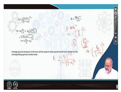
So if contact pressure is p<sub>i</sub>+p<sub>c</sub> then the sinkage we can calculate,
