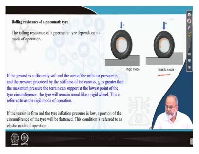
Then, in case of a pneumatic wheel, it behaves in two different modes during operation, the first mode is in rigid mode, the second mode is in elastic mode. Rigid mode means the rolling resistance, the tyre will simply sink into the soil, it is not flattened.
