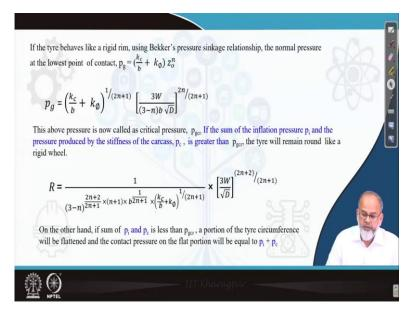
So if the tyre behaves like it is a rigid rim then you have to use the same Bekker's equation what we have utilized in case of a rigid wheel and the normal pressure at the lowest point of the tyre is given by
