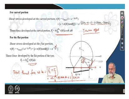
So, for the curved portion, again we have to find out what kind of soil is there? If it is a loose soil, if it is a organic terrain or if it is a compact sand then we have three different kinds of relationship available. So, based on that, we have to find out the relationship between shear stress and shear displacement. So, in this case, I have taken the loose sand where,
