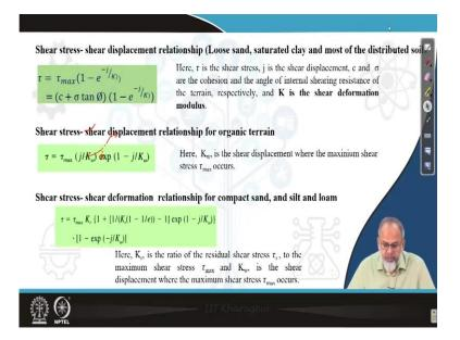
So, in nature what we have observed is there are three different categories of relationship available are found. One is related to loose soil, the other one loose soil or saturated clay and in disturbed soil and the other one is in organic terrain, then the third one is in compact sand silt and loam. So, these are the three relationships which we have discussed earlier and the relationship in these three conditions like loose sand, saturated clay,
