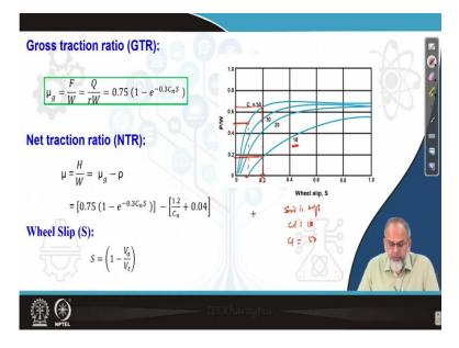
The second equation which he developed is related to gross traction ratio. So, gross traction ratio means if the ratio of the tractive force which is developed at the contact patch divided by the dynamic weight coming in the wheel. So, in other words, we can replace F with Q/r. So, Q/r, Q is the torque which is acting on the axle, r is the rolling radius. So, that way thrust×radius will give you Q. So, we have replaced F that is tractive force with F×r, tractive force into rolling radius as Q.
