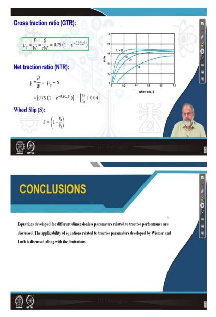
Now, looking at the limitations of Wismer and Luth equation, the motion resistance ratio as I told in the beginning, it does not contain a slip term. So, that is why it will predict the same value of motion resistance for a towed wheel as well as a powered wheel. Applicability of equation which is developed by Wismer and Luth is only limited to b/d ratio as 0.3,  $\delta$ /h ratio as 0.2, and r/d ratio as 0.475. So, these are the limited applicability.
