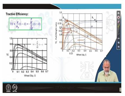
So, if you look at this curve, so, you are nearly when the soil is hard that means the mobility number is 80 you can see we are reaching to a peak here, and when the mobility number is 40 we are reaching to a peak here, when the mobility number is 20 we are reaching the peak here.
