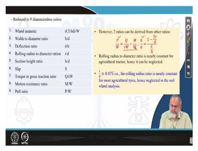
Out of these 9 dimensionless ratio variables, he identified as wheel numeric, CIbd/W, width to diameter ratio (b/d), that means section width to wheel diameter, deflection ratio ( $\delta/h$ ), rolling radius to diameter ratio (r/d), section height ratio (h/d), that means section height by overall diameter, slip, torque or gross traction ratio (Q/rW), motion resistance ratio (M/W) and pull ratio as P/W. So, these are the 9 dimensions ratio variables he identified.
