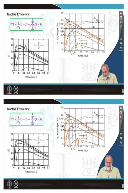
Next thing is tractive efficiency. Once you derive motion resistance, coefficient of traction, then we tried to find out what is the expression for tractive efficiency. The expression remains same that means output power by input power. And it is a function of slip So,
