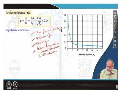
So now, let us see what is the equation which is developed for motion resistance ratio, which is denoted as  $\rho$  and this is equal to M/W and
