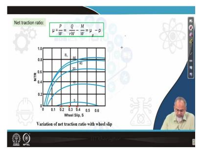
Then he derived coefficient of traction or net traction ratio which is
