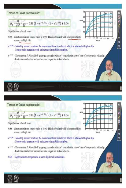
Then the equation which he developed is torque or gross traction ratio. This is written as Q/rW, Q is the torque and r are the rolling radius, W is the dynamic weight. So, in other words you can write F/W that means tractive force divided by the dynamic load
