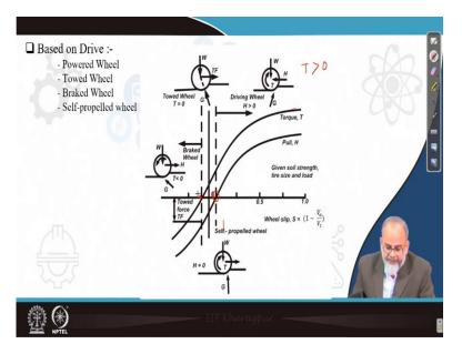
The wheel can be classified as powered wheel, it can be classified as towed wheel, it can be classified as braked wheel or it can be classified as self-propelled wheel. So, these classifications are based on power and torque characteristics of the tyre versus slip. Now, what is a powered wheel? When a wheel is provided with a torque that means initiate with a torque then it is powered.
