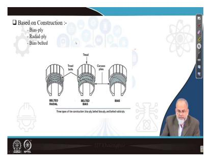
Now, based on construction, the pneumatic wheels can be called as a bias tyre or bias belted tyre or radial tire. Commonly, the bias belted are being used by the tractor manufacturers either bias tyre or bias belted tyre and nowadays radial tires are coming into picture, the only advantage in case of radial tyre is, it will have more sidewall deflection, so contact area is more. That is the main advantage over belted or bias belted tyre.
