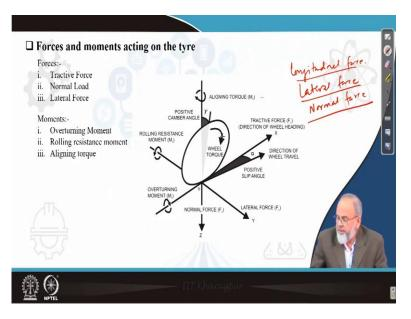
Now, the next important thing is what are the forces of moments acting and how do we represent it, that is important. So, to describe the forces and moments acting on a wheel, we have to take the help of a axis system which has been recommended by Society of Automotive Engineers. Where, there will be three forces, three moments and this will be indicated in this figure which you can see on the right side.
