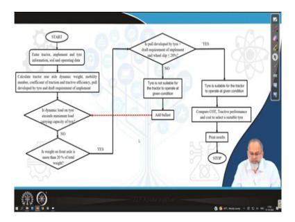
We have to calculate the rear axle dynamic weight then based on that and using Brixius equation you have to find out different traction parameters like COT, CRR then tractive efficiency then you have to calculate from COT what is the pull available and then what is the draft required by the implement. So, once all these parameters are calculated, next thing is the dynamic weight which is coming at the rear axle and part half of that will come on each of the wheels.
