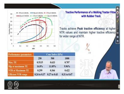
Let us see, now the plot, the different plot where we will see the effect of all the parameters, performance parameters that means in y axis we have traction ratio and slip ratio and on the x
