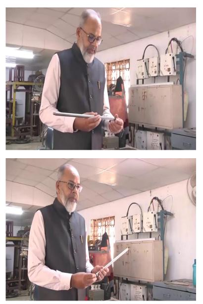
There is a cone penetrometer meter which has been, the cone has been removed from this shaft to which it will be attached. This cone along with this shaft has to push, has to be pushed into the soil of the soil bin, and how much force we are applying that has to be recorded. And the base area of this cone is 3.23 square centimeter and the angle of the cone is 30°.
