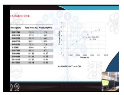
Again, we try with another diameter plate which is 35 centimeter we got the sinkage data here, we got the force data and then force divided by the area of the plate, so, that will give you the pressure data. So, now, we try to plot pressure versus sinkage. So, what we observe here is, again a power equation which will be a best fitting the observed data points. So, the pressure is equal to  $684.89 \times \text{sinkage}^{0.7661}$ .
