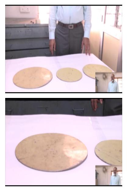
It is a rectangular plate or a circular plate which simulates the contact area of a tyre and that has to be forced to enter into the soil. So, what you are going to measure is the force which is required to press it and what is the corresponding sinkage. So, once you know the force, force divided by the area, area of the plate that will give you pressure. So, and the corresponding sinkage will try to measure, so, I will try today with the 3 plates of different diameter.
