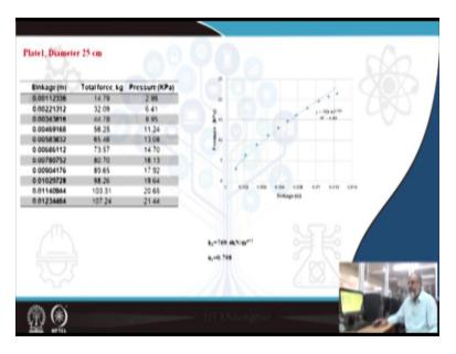
Now, the data which you obtain related to plate 1, that is diameter 25 centimeter, this is the sinkage values, these are the corresponding force values and then force are converted to pressure by dividing its area ( $\pi r^2$ ). So, these are the pressure data which you got. Now, you try to plot these pressure data against the sinkage data. So, sinkage we have taken on the x axis and pressure you have taken y axis.
