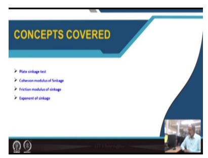
Where I will try to clear the concepts like what is the setup which is used for measuring plates sinkage, and then we will try to find out what is the Cohesive modulus of sinkage, frictional modulus of sinkage, exponent of sinkage. And these parameters are important related to and they are related to bearing strength of soil. So, that is why, we are interested in measuring these, these parameters.
