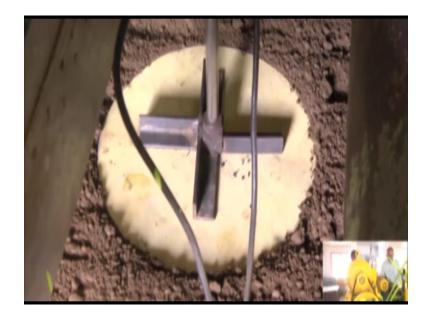
I will now show you the setup which is used for measuring the pressure of a pressure required to place a plate into the soil. The setup comprises of a plate which is kept over the soil surface is the plate which has a diameter of 30 centimeter. Then this has to be pressed using a shaft, this shaft is connected to the hydraulic cylinder, this the hydraulic cylinder. So, in between the shaft and the hydraulic cylinder, there is a load cell that is going to measure how much force you are applying.
