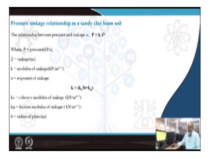
In a pressure sinkage test what we are measuring is, how much pressure we required to force a plate. Plate could be a rectangular plate, plate could be circular plate, and that should simulate the contact area of a tyre. Now, it is better to take a circular plate because when you apply a load, it becomes uniformly distributed, if you take a rectangular plate, the corners are dead points. So, that is why pressure is not uniformly distributed.
