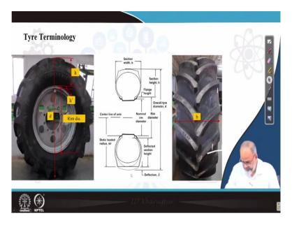
Now, after knowing in details about the constructional features, the next thing is, what are the different terminology associated with a tyre whether it is a bias ply tyre whether it is a belted tyre whether it is a bias belted tyre. These terminologies remain same; same in the sense it has section width, it has section height, it has overall diameter. So, all those things we are going to discuss in detail.
