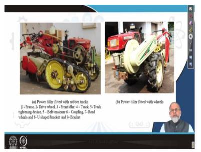
So, to carry out this kind of study, what we have done is, a power tiller is fitted with a track, rubber track and the power tiller is fitted with a normal wheel and their performance will be compared when they are operated under the same operating conditions.
