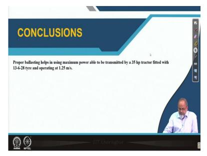
So, this will give you a more or less an idea how to go for ballasting two wheel drive tractor to get the maximum output from the tractor. That is all. Thank you.
