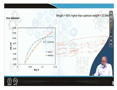
So, look at these figures now, so, that itself indicates what is exactly happening. So, you are closer to 14 kW, the maximum power where, which a tractor is able to transmit. Whereas in case of over ballasting condition, we are developing, only we are utilizing only 10.4 kW. We are supposed to get 14 kW, but we are not developing 14 kW. There is a loss. At under ballasting conditions, we are only utilizing 6 kW. we are supposed to utilize 14 kW.
