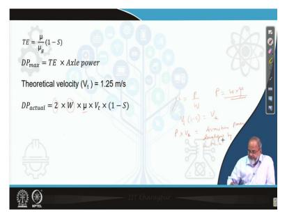
And tractive efficiency is nothing but the axle power by, sorry drawbar power by axle power or in other words,
