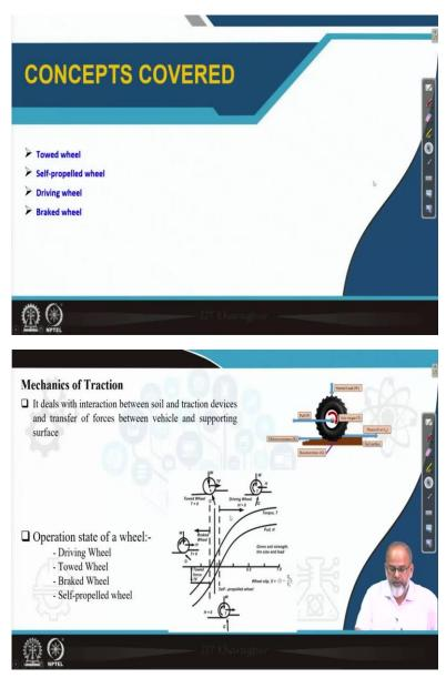
So as you know, the concepts which I am going to cover the towed wheel, self-propelled wheel, driving wheel, then mechanics of traction. As you know mechanics of traction is nothing but interaction between soil and the traction devices and the transfer of forces
