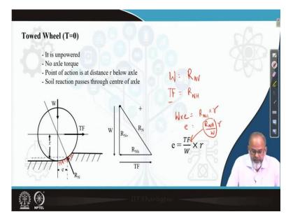
So, when a vehicle is moving, it is applying a load to the wheel at the axle and at the same time the soil will try to apply the reaction force to the wheel at the interface, interface means the soil-wheel interface. So load, from the vehicle will act on the axle, the reaction from the soil will be acting at the soil will interface.
