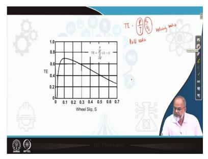
Now, tractive efficiency. Tractive efficiency is defined as the drawbar power to axial power. So, I have given the expression for that
