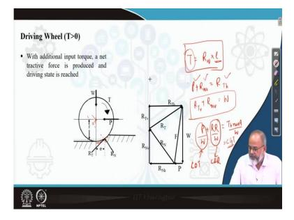
Now, we will move to the powered wheel or the driving wheel. Here two things, we will be seeing, one, there will be torque which is denoted as T and there will be a pull applied P. So, torque is indicated here, torque, and there is a pull here. Now, because of the torque there will be again shearing forces acting at the interface and the resultant of that shearing force is RT and the soil reaction RN coming from the wheel to the ground and W is acting downward.
