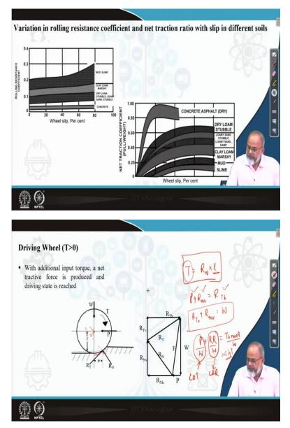
Now, let us see what are the different performance parameters now, how it is varying with slip. As you discuss that performance parameters are your coefficient of traction, coefficient of gross traction, tractive efficiency, then power delivery efficiency, these are the performance parameters. So, now we will see how the coefficient of rolling resistance is varying it wheel slip.
