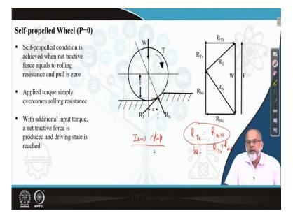
Now, if you look at this figure, you can see, there is a torque acting, weight acting on the wheel and because of the torque that we will be shearing action, so a tangential force will develop on the interface and the resultant of that tangential force is denoted as RT. So, at the interface there will be two kinds of forces acting, one is RT, the other one is RN. RN is the soil reaction, which is radial soil reaction.
