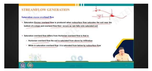
So, this is a pictorial view of the two types: first, infiltration excess overland flow. Excess water that cannot infiltrate ponds on the soil surface and eventually starts to flow down slope across the soil surface. Here, precipitation is occurring, and of course, some water infiltrates, and then as a thin layer, it starts moving on the soil surface. In the case of saturation excess overland flow shown here, subsurface flow returns to the surface when the capacity of the soil to transmit
