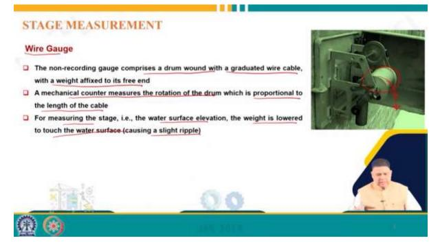
Another type of non-recording gauge could be a wire gauge, which comprises a drum wound with a graduated wire cable with a weight affixed to the free end. So, you can see here there is a drum here on which this wire cable is wound, and of course, at the loose end, we fix a weight.
