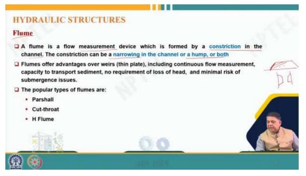
Moving on to the third type of hydraulic structures, which are flumes. Flumes serve as flow measurement devices and are created by a constriction in the channel. This constriction can be achieved through channel narrowing, a hump, or both. Therefore, if a channel is present, it can include a hump-like structure or narrowing in its width. This constriction can be achieved either by raising the channel bed with a hump or by narrowing the channel width.
