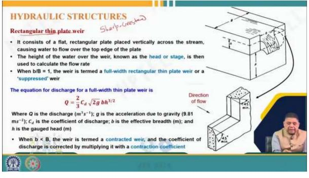
The width of the rectangular channel and the width of this rectangular thin plate weir are the same, then it is referred to as a full width rectangular thin plate weir or it is also referred to as a suppressed weir.
