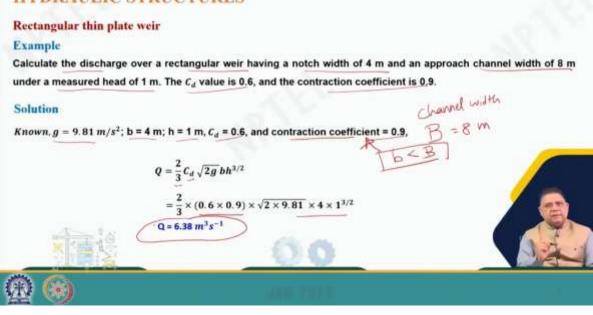
Just taking a simple example, calculate the discharge over a rectangular weir having a notch width of 4 meters and the approach channel width of 8 meters under a measured head of 1 meter. The cd value is 0.6, and the contraction coefficient is 0.9. So, these are the known values we already know: b is given, h is given, cd is given, and the contraction coefficient is given. Of course, another thing which is given is the channel width, that is, channel width, which is 8 meters.
