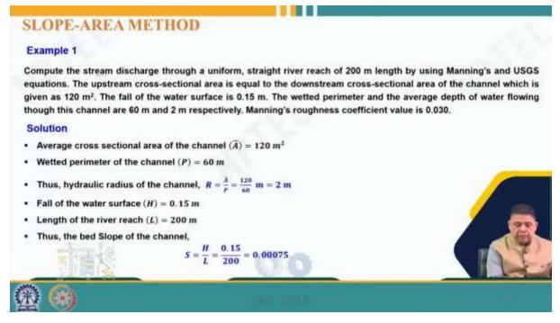
So, it is a uniform section, the fall of water surface is 0.15 meters, the weighted perimeter, and the average depth of water flowing through this channel are 60 meters and 2 meters respectively, and Manning's roughness coefficient value is 0.03. So, it is a uniform cross-section, and that means Manning's equation can be straight away used. So, the average cross-sectional area is given as 120 square meters, the weighted perimeter is given as 60 meters.
