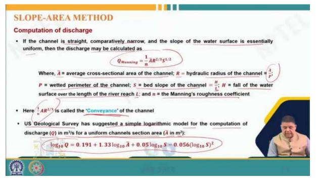
So, where the flow is under gravity, then only this method is applicable. Now, coming to the computation of the discharge, if the channel is straight, comparatively narrow, and the slope of the water surface is essentially uniform, then the discharge may be calculated using Manning's equation.
