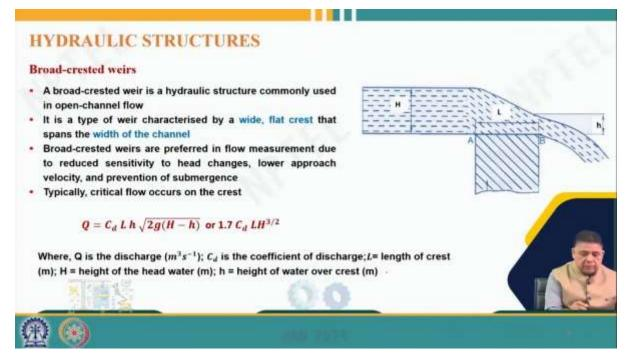
So, as the water level rises, the velocity in this portion becomes subcritical. Then, when the crest is reached and beyond it, there is a free-flow condition. It is expected that the velocity will increase beyond the crest, becoming supercritical. This is why a critical velocity is anticipated over the crest. Thus, there will be a critical velocity. This critical depth is essentially measured at the crest. The formula that can be used for critical flow is:
