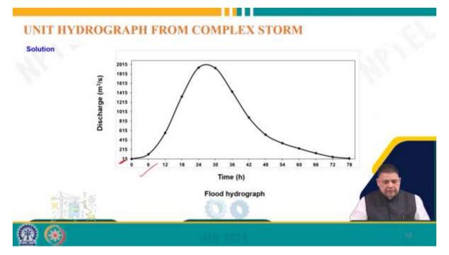
Because it is 15, so it is not starting at 0, but we have started the scale from 15. So, they do not get confused; there is a base flow component of 15 and so on throughout 15, 19, 17, 19, and so on and so forth. So, this is how we can get the unit hydrograph from complex storms.
