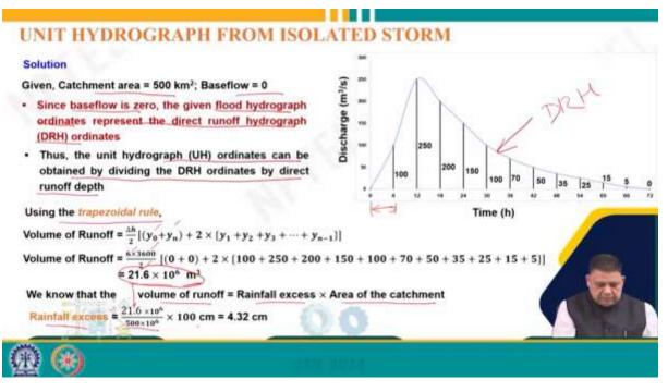
Here we have been given that the catchment area is 500 square kilometres and the base flow is 0. Since the base flow is 0, the given flood hydrograph ordinates basically represent the direct runoff hydrograph because we deduct the base flow, but since the base flow is not there (it is 0), whatever is given to us is a direct runoff hydrograph, and this is what we have plotted here.
