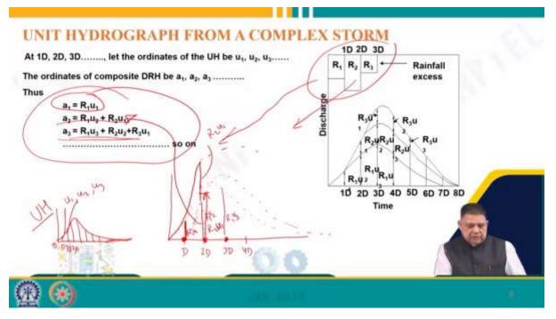
But let us try to understand this, basically what happens is that suppose you have a unit hydrograph, say U, its ordinates are U1, this is the unit hydrograph. Then its ordinates at different times are U1, U2, U3, U1, U2, U3, these are the ordinates of this unit hydrograph which we are trying to find out. I am just trying to explain it in the converse of the problem we are trying to handle.
