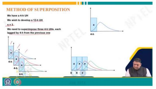
So, coming to the method of superposition, we have a 4-hour unit hydrograph, and we wish to develop a 12-hour Intergraph, that means n is equal to 3, D-hour to ND-hour, we said n equal to 3. So, we need to in that case, we need to superimpose 3 4-hour unit hydrographs each lagged by 4 hours from the previous one.
