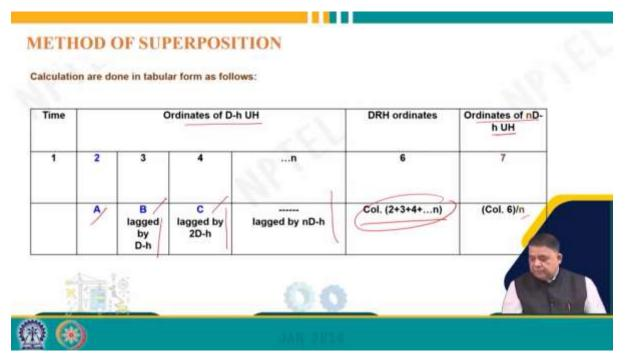
So, calculations can be done in tabular form, just like we saw also. So, the ordinates of the DRH hour, a b lagged by 4 d hour c lagged by 2 d hour and n lagged by n d hour, then the sum of all these ordinates will give us DRH ordinates, and then because it is an n d hour unit hydrograph, ordinates will be this sum divided by the value of n. So, if n was 3, that is why we superimpose 3-unit hydrographs.
