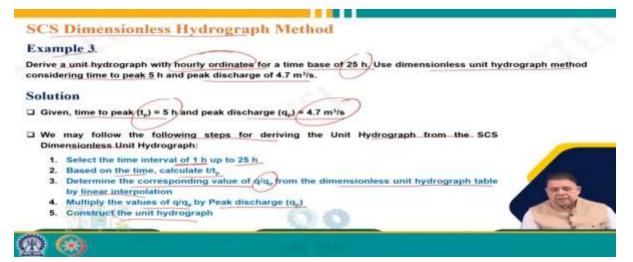
Now, we will take an example here, example 3. So, to see the application of the SCS dimensionless hydrograph method, derive a unit hydrograph with hourly ordinates for a time base of 25 hours, and use the dimensionless unit hydrograph method considering time to peak at 5 hours and peak discharge of 4.
