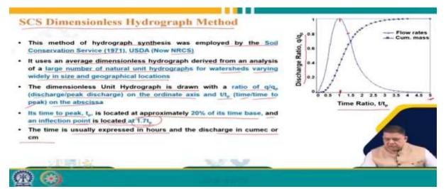
Now, we get into the SCS dimensionless hydrograph method, which is the other method, and this method of hydrograph synthesis was employed by or developed by the Soil Conservation Service. They developed this in 1971, and SCS, we know that now is known as NRCS, which is the Natural Resource Conservation Service, and of course, it belongs to USDA, US Department of Agriculture.
