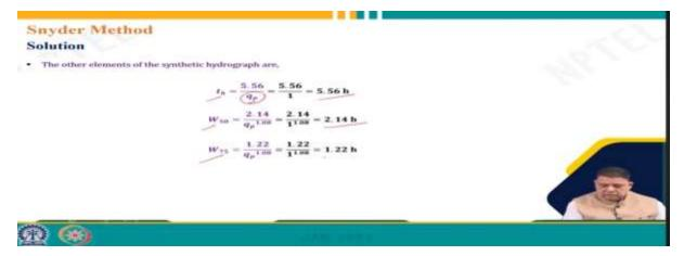
Now, other elements are that like  $t_b$ ,  $W_{50}$ ,  $W_{75}$ , knowing  $q_p$ , we can calculate this, and then we can  $q_p$  that is, we have to use the in cumecs per square kilometer as per this relationship. So, putting the values, we get  $t_b$  equal to 5.56 hours,  $W_{50}$  is 2.14 hours, and  $W_{75}$  is 1.22 hours. So, now, that means, we know everything, and knowing that, we can plot the hydrograph quite easily.
