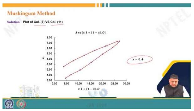
So, like here, we are plotting column 7 versus column 11, that means, for x equal to 0.4, we can start with x equal to 0.1, it does not matter, because you have to plot each. So, this is what we get. You see we are getting a loop, but it is quite a gap, a broad gap, between two tails.
