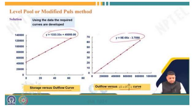
and so, this is the equation we have; this is the curve we have developed, and these are the equations we have developed. So, on the left side, we have the storage versus outflow curve,
