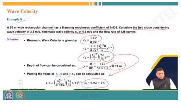
So, wave velocity v will be frac {q} {a cdot b cdot y}. So, q is known to us, b is known to us, y we have calculated. So, that comes out to be 1.56 meters per second and the kinematic wave celerity  $C_k$  we know is that frac {1} {b} cdot frac {dq} {dy} and that means, frac {1} {b} cdot frac {dy} {dy} of this value q value already we know, and which ah on ah ah which comes out to be frac {a cdot h} {n cdot left(frac {5} {3} cdot y right)^{5/3}}.
