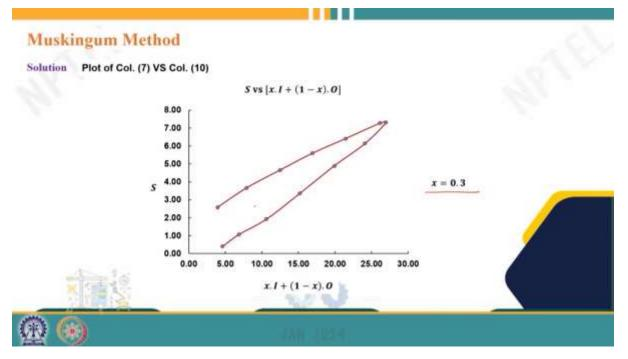
Then this one is a plot we get for x equal to 0.3, a little bit narrower than 0.4,
