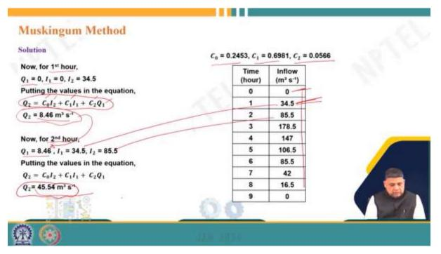
Then, of course, we need to route the flow. So, our  $C_0$ ,  $C_1$ , and  $C_2$  are known, and the inflow hydrograph values are given to us. So, for the first hour, we do not have any information. Also, we are assuming Q\_0 is 0, and I\_0,  $I_1$  is 0, and  $I_2$  is 34.5. So, putting the values in this equation
