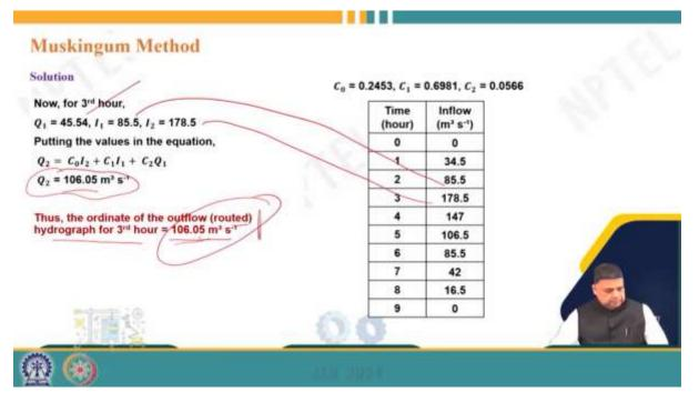
So, here  $Q_1$  will become 44.54, then 85 will become  $I_1$ , 178 is  $I_2$ , and knowing the values of  $C_0$ ,  $C_1$ ,  $C_2$ , we can calculate  $Q_2$ , that is, at the end of the time interval, at the third hour, which is the third routing time interval, the third hour, the ordinate we are getting is 106.05 cubic meters per second. So, that is the answer, that the ordinate of the outflow routed hydrograph for the third hour is 106.05 cubic meters per second.
