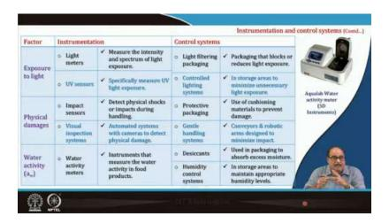
Then for even instruments for exposure to light, there are light meters or UV sensors can be used. Light meters which measure the intensity and spectrum of light exposure ok.
