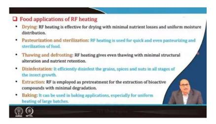
Radiofrequency heating or radio frequency waves are employed as a pretreatment for extracting bioactive compounds with minimal degradation. It can be used in baking applications, especially for uniform heating of large batches, etcetera.
