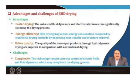
Regarding the advantages and disadvantages of EHD drying, the advantage is the faster drying process; the enhanced fluid dynamic and electrostatic forces can significantly speed up the drying process. Again, it is also an energy-efficient process, and it may reduce energy consumption compared to the traditional drying method by improving heat transfer and moisture removal and product quality. Drying using this technology results in a good
