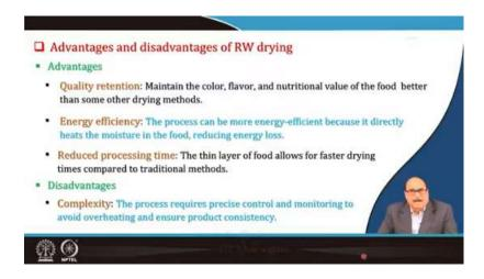
It has good energy efficiency; the process can be more energy efficient because it directly heats the moisture in the food, reducing energy loss. There is a reduced processing time. The thin layer of food allows for faster drying times than traditional methods. Its disadvantage, however, is the complexity of the process. The process requires precise control and monitoring to avoid overheating and ensure product consistency.
