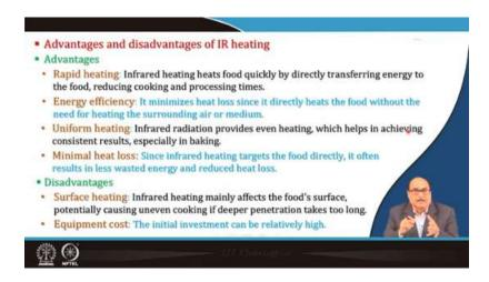
Since infrared heating targets the food directly, it often results in less energy waste and reduces heat loss. The disadvantages, however, are that infrared heating mainly affects the food surface, potentially causing uneven cooking if deeper penetration takes too long. So, the equipment cost and the initial investment can be relatively high.
