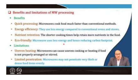
Benefits and limitations of microwave processing: The benefit is quicker processing. It can cook foods much faster than the conventional method. It is an energy-efficient process; it uses less energy than conventional ovens and stoves, resulting in better nutrient retention because of the shorter cooking times; it is an eco-friendly technology in which microwaves use less energy and hence reduce the carbon footprint. The limitation, however, is that
