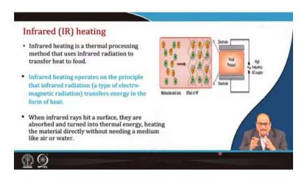
So, you can see that molecule and the effect of radiation on the food product, which directly heats internally. So, there are two electrodes, and the food is placed between these two electrodes.
