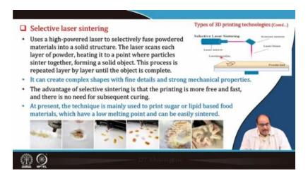
Selective laser printing uses a high-powered laser to selectively fuse powdered materials into a solid structure. There is a sensitive laser sintering process. Here, the scanner system is present. So, the laser beam is coming, and there is a leveling roller here. The
