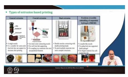
So, the different types of extrusion-based 3D printing may be general extrusion, coaxial extrusion, dual extrusion or freeform reversible embedding of suspended hydrogel that is FRESH extrusion process.
