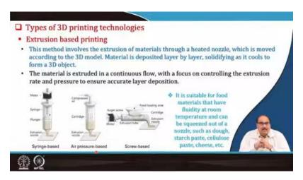
So, let us discuss what are the different types of 3D printing technology and first which is the most commonly used technology for the 3D printing of the food materials is the extrusion-based printing. So, this method basically involves the extrusion of material through a heated nozzle, which is moved according to the 3D model that you have already selected and decided. And then material is deposited layer by layer solidifying as it cools from a 3D object.
