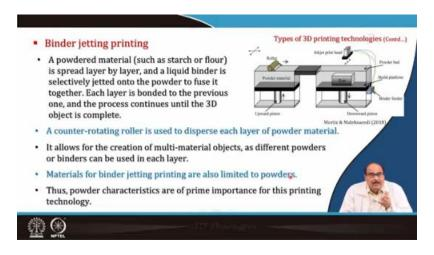
Now, the other type of food printing. 3D printing machine is the binder jetting printer or binder jetting printing. So, here as you can see in this figure, a powdered material such as starch flow or such other material is sprayed layer by layer and a liquid binder is selectively jetted onto the powder to fuse it together. So, each layer is bounded to the previous one and in the process that the process continues until the 3D object is complete.
