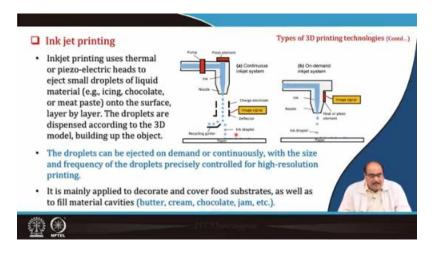
Inkjet printing uses thermal or piezoelectric heads to eject small droplets of liquid materials, for example, icing, chocolate, or meat paste, etc., onto the surface of the food material layer by layer. The droplets are dispersed according to the 3D model of the object. This can be done by ejecting droplets on demand with an on-demand inkjet system, or they can be injected continuously, with the size and frequency of the droplets precisely controlled for high-resolution printing.
