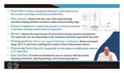
Then there are feed rollers, as you have seen in the earlier systems. These rollers assist in feeding the filament or food materials onto the extruder or such other system, ensuring a steady and controlled flow. There are flow sensors that monitor the flow rate of the material being extruded, helping maintain consistent output and preventing clogs. Pressure regulators control the pressure at which the material is extruded or printed or shaped, ensuring smooth and even deposition.
