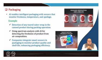
Then, in the packaging, AI enables intelligent packaging with sensors that monitor freshness, temperature, and spoilage. For example, these systems can detect torn outer wraps in the canned product during packing operations. Spectrum analysis with AI is used to detect the freshness of the product from the air composition. A few companies integrate smart sensors in packaging to monitor product quality. Shelf life enhances packaging
