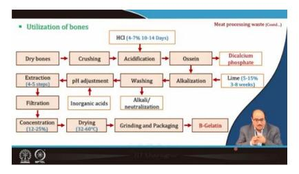
So, even the bones can also be utilized for the preparation of dicalcium phosphate or for beta gelatin, etcetera. And the process is shown here: dry bones, crushing, acidification with the help of hydrochloric acid (4 to 7 percent) for 10 to 14 days, then alkalization
