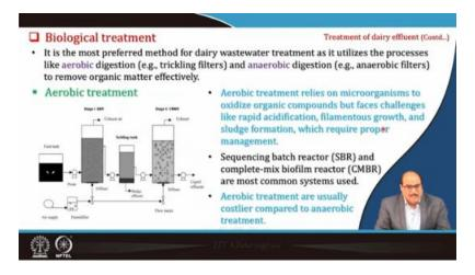
Then biological treatment, it is the most preferred method for dairy wastewater treatment as it utilizes the process like aerobic digestion using trickling filters or anaerobic digestion using anaerobic filters etcetera. And in this way either by aerobic methods or by anaerobic methods the organic matters are most effectively utilized or removed. So, in the aerobic methods as you can see here in this diagram, that this method mainly relies on the
