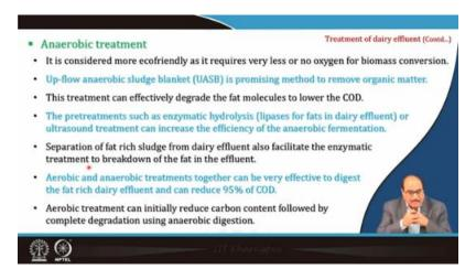
Anaerobic treatment is considered more economical as it requires very less or even no oxygen for biomass conversion. Up-flow aerobic sludge blanket that is UASB is a promising method to remove organic matter. This treatment can effectively degrade the fat molecules to lower the COD value. The pretreatments such as enzymatic hydrolysis by using lipase etcetera for the hydrolysis of fats are using is treating it with the ultrasounds. This can increase the efficiency of the anaerobic fermentation.
