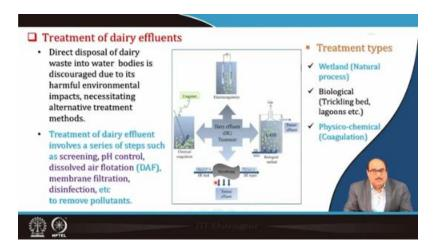
So, it becomes a very very important one should have a proper mechanism for the effluent treatment dairy effluent treatment. So, what are the different there are different approaches different method for the treatment of dairy effluent. that like direct disposal of the dairy waste water into water bodies is discouraged. mainly due to it is a harmful environmental impact, necessitating alternative treatment method that is it should not be directly exposed to environment or in the water body.
