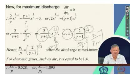
2 by gamma plus 1 to the power gamma by gamma minus 1, right? That is the pressure ratio. Now, mind it here, our pressure ratio is outlet, that is tip to the inlet, that is more, right. So, that is why it is coming from high to low. That is why we gave the example of refrigerant.
