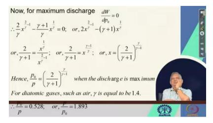
A diatomic gas has a gamma, which is the heat capacity ratio  $C_P$  over  $C_V$ , of 1.4, right. So, therefore, if it is a diatomic gas, then we write  $P_o$  over P to be equal to 0.528,  $P_o$  by P to be 0.528, because  $P_o$  by P is equal to 2 by gamma plus 1. to the power gamma by gamma minus 1. Now,  $P_o$  by P is equal to 2 by 1.4 plus 1 to the power 1.4 divided by 1.4 minus 1. So, this is equal to 2 by 1.4 plus 1, which means 2 by 2.4
