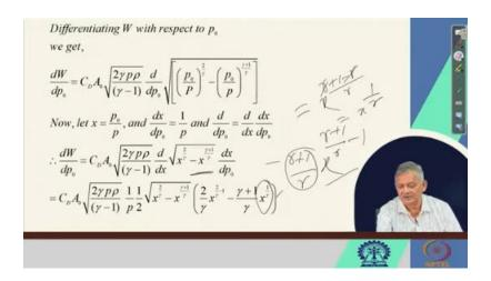
into 2 by gamma x to the power of 2 by, sorry, x to the power of 2 by gamma minus 1 minus gamma plus 1 by gamma to the power of x to the power of 1 by gamma, right. This is our  $dW / dP_o$ . Now, the rate of change of W, discharge, right. If that becomes 0, that is  $dW / dP_o$ , if it becomes 0, right. So, when will it happen?
