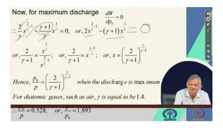
So, that correction, please do. Now, what is it that we have? 2 x to the power 2 by gamma minus 1 minus gamma plus 1 into x to the power 1 by gamma, right? Therefore, we can write 2 by gamma plus 1 that is equal to x to the power 1 by gamma. Over x to the power 2 by gamma minus 1, right? Gamma plus 1.
