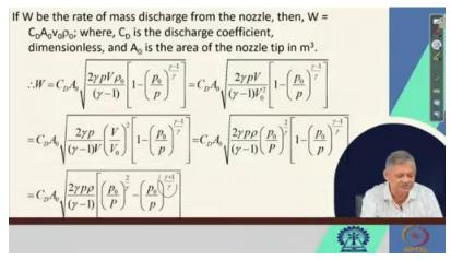
W is  $C_D A_o 2$  gamma P rho by gamma minus 1 into  $P_o$  by P to the power 2 by gamma minus  $P_o$  by P to the power gamma plus one How gamma plus 1 came, that also we have said, right? Just for a recapitulation, that this  $P_o$  by P to the power 2 by gamma is put inside this bracket. So, it became  $P_o$  by P to the power gamma 2 by gamma into 1. Right, and then this  $P_o$  by P here it is getting multiplied.
