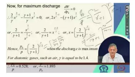
So, this we have to keep in mind for maximum discharge, the pressure ratio that is tip to inlet is 0.528, or the inlet to the tip is 1.893. With this, we have come to the end of this
