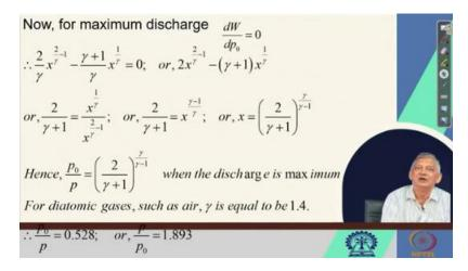
What could be 0?  $dW / P_0$  is 0, then what could be 0, right? This cannot be 0, where is that, ok. You see, this cannot be  $C_D$   $A_0$ , it cannot be 0 because  $A_0$  is a definite number,  $C_D$  is also a definite number, this cannot be 0. 2 gamma P rho are all some positive quantities.
