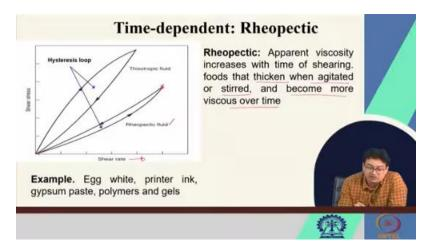
Because of the change in the molecular structure or structural changes again. What are some examples? Egg white, printer inks, gypsum paste, polymers, and some gels. So, if you have this kind of product, the more you agitate or mix, it may become more viscous. That means the apparent viscosity increases over the time period.
