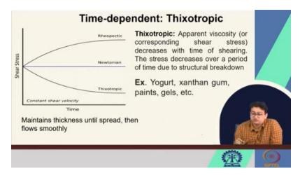
So, we have a food product now that is actually subjected to a shear. So, the longer you shear the apparent viscosity it will change and eventually it will decrease ok. Therefore, the stress also decreases over a period of time due to the structural breakdown ok. So, what happens? So, initially
