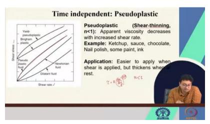
Because it has got some yield shear stress, that means it is behaving as a pseudoplastic. But to make it flow, we have to apply some initial force. That means the initial shear stress has to be applied. What are the examples? Ketchup, sauce, chocolate, nail polish, some different kinds of paints, inks.
