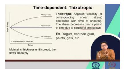
And if you look at the picture, here in the x-axis we have time, and here we have the shear stress, ok. The rheopectic one, sorry, the thixotropic one looks like this. So, it is starting from here, the shear stress over here, and eventually it is decreasing as the time progresses. This one is Newtonian. It is giving us a straight line parallel to the x-axis, ok.
