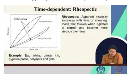
On the x-axis, we have the shear rate. So, we are slowly increasing the shear rate, let us say up to a maximum value over here. In the rheopectic, initially, the apparent viscosity was some over here. Eventually, with time of shearing, it is increasing. That means, say, if you have any food you are mixing.
