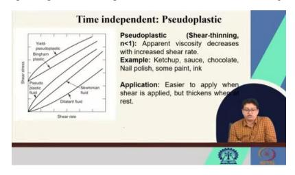
So, if you recall, we had an equation of du dui to the power n. So, this is the flow behavior index. In pseudoplastic, shear thinning behavior has n less than 1, ok? That means apparent viscosity decreases with an increase in shear rate. So, here, if you look at this picture, this graph has the shear rate on the x-axis and shear stress over here.
